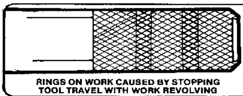
Figure 7-94. Rings on a knurled surface
